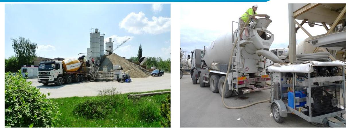
filling of the drum by technical foam and cement grout, homogenization of fresh mixture during the transport, screw or piston pump on site
